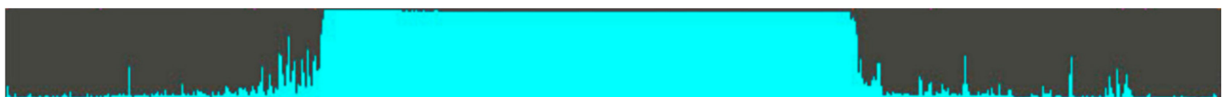
Figure 10. The measured intensity of one profile on a shiny smooth surface. Points in the laser line are no longer detected on the left and right side because of low laser intensity.
