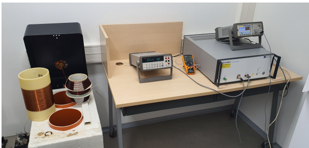
Fig. 2: Propopsed and constructed experimental setup showing the applicator used in preliminary experiments and the newly designed applicator.
