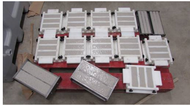
Fig. 1: Test specimens cast into the polypropylene moulds.
