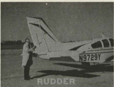
35. This is the rudder that makes the airplane go left and right.
