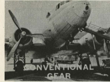
43. This is another kind. It is called conventional landing gear. What is the difference?
