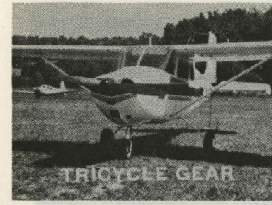
42. This is one kind of landing gear. It is called tricycle gear.
