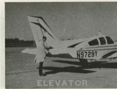
36. This is the elevator. It makes the plane go up and down.
