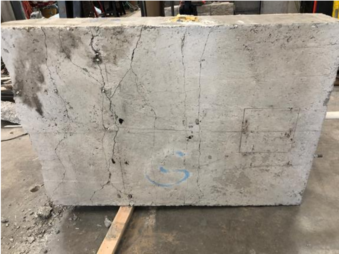
Figure 5-24 Face of GFRP Reinforced Slab After Failure
