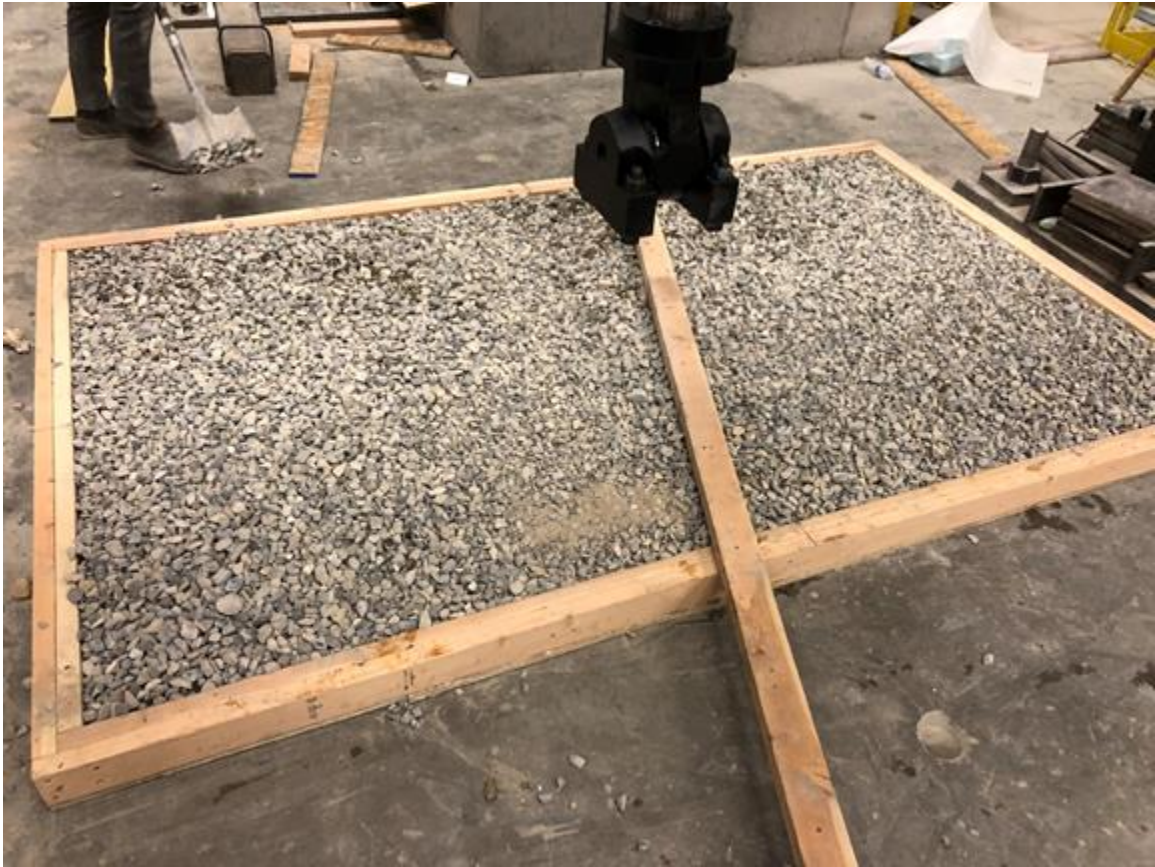
Figure 3-4 Gravel Containment Box
