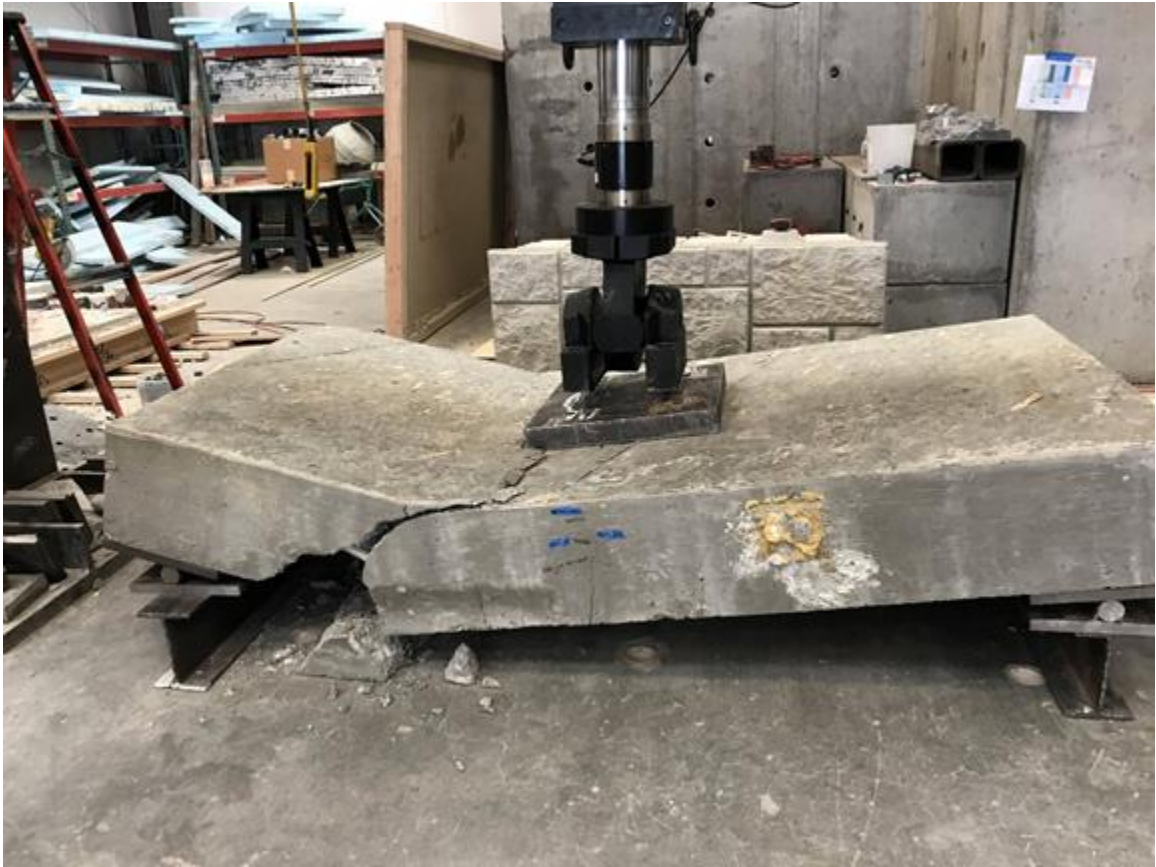
Figure 5-21 GFRP Catastrophic Failure
