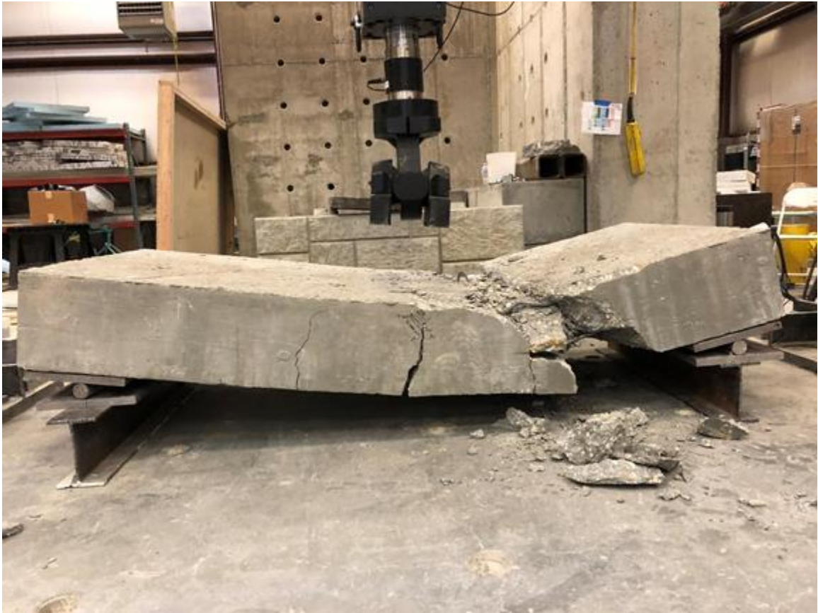
Figure 5-11 panel with Steel reinforcement Catastrophic Failure
