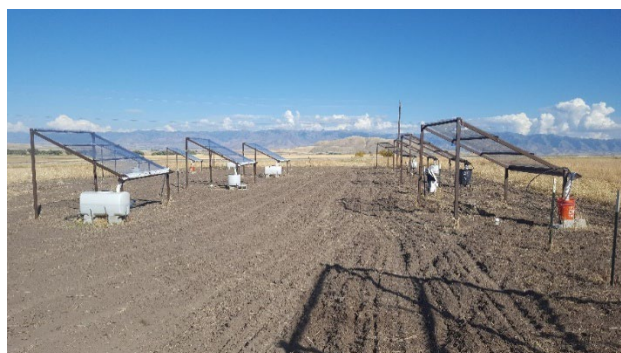
Figure 3.2 Shelters ( 2.1 \times 2.5 m) were used to redistribute rain and snow as fewer, larger events at a dryland agriculture site, Utah, USA. Two of three rows of plots are visible in the photograph.
