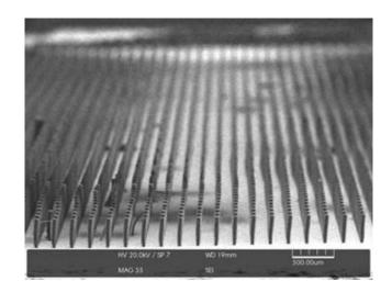
Figure 4.18 More than 2000 micropillar array in a one-inch glass.
