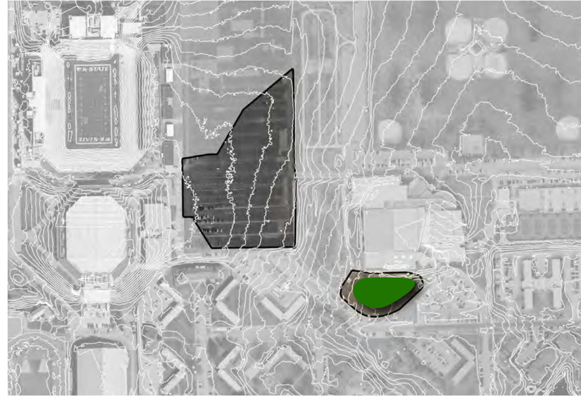
Figure 7.14. East Stadium Focus Area Proposed Bioretention.
