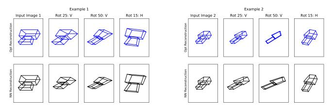
Figure 1: Two examples of 3D shape reconstruction by the NN and by an explicit optimization (Opt). The input image is on the left. The additional 3 views show the reconstructed shape after rotation around vertical and horizontal axes.
