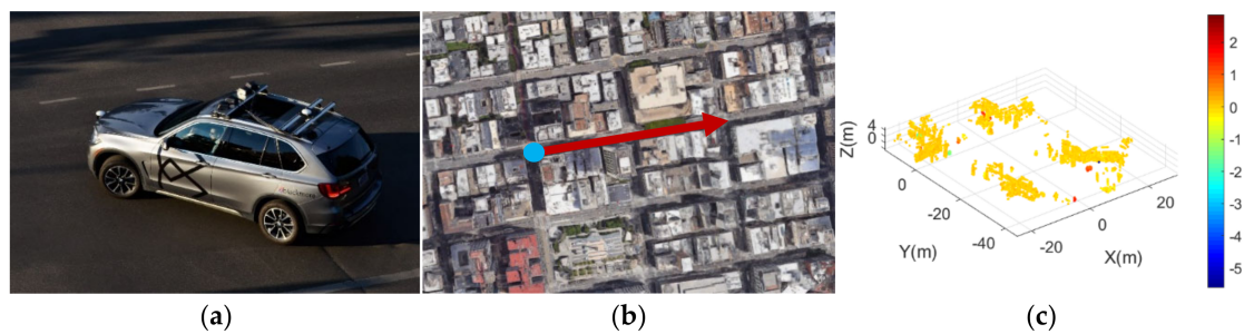
Figure 1. (a) The Doppler LiDAR system; (b) the test site (blue dot: the sensor; red arrow: driving direction); (c) one frame point cloud color coded by absolute radial velocity (unit: m/s).
