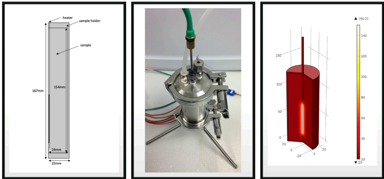
Figure 2. Schematic of R22B10T1 case: TPCell instrument with the center heater (left), and simulation of the center heater with product (right).
