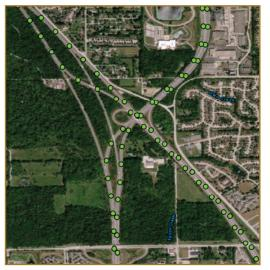
Mapping of 0.1-mile reference points along segments of interstate using GIS tool.
