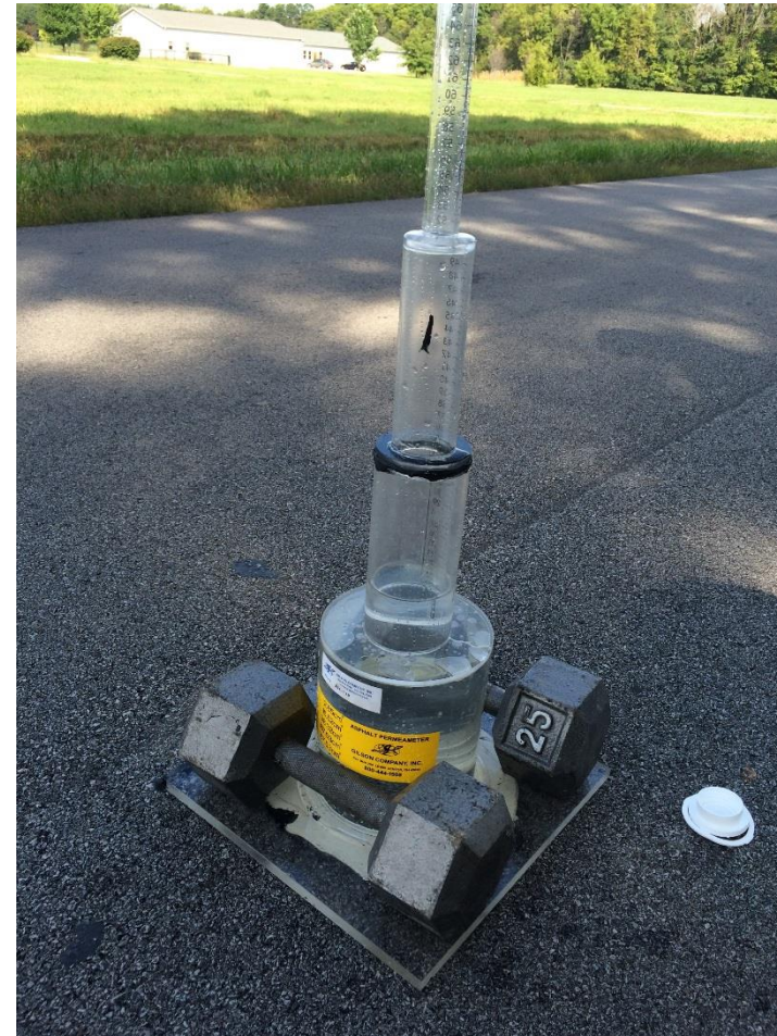
Falling head permeameter
