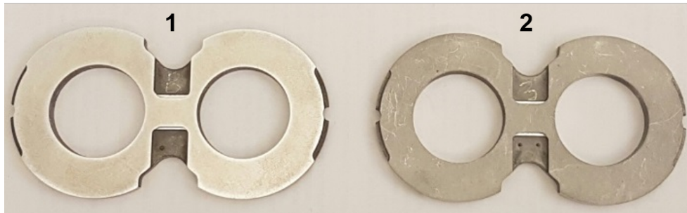
Figure 5.1. Sample lateral plates belonging to the same reference EGM with varying surface roughness.
