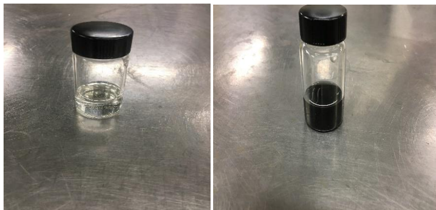
Figure 3-18- the PVDF solution (left) and PVDF-GO solution(right)
