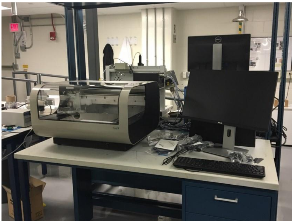
Figure 4-4- Dimatix material printer (DMP-2850) with a piezo inkjet cartridge.
