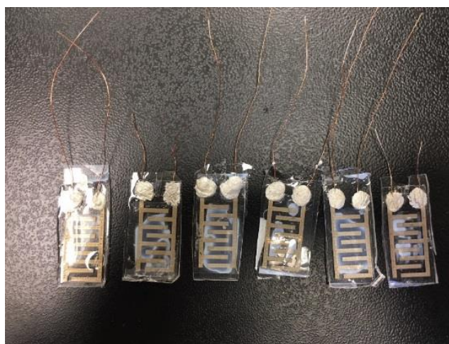
Figure 4-8- Multiple piezoelectric PVDF devices made by inkjet printing process
