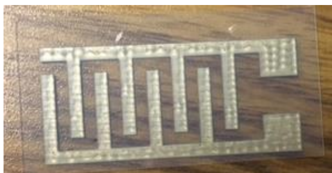
Figure 4-6- The pattern of IDE electrode using the inkjet printing process.
