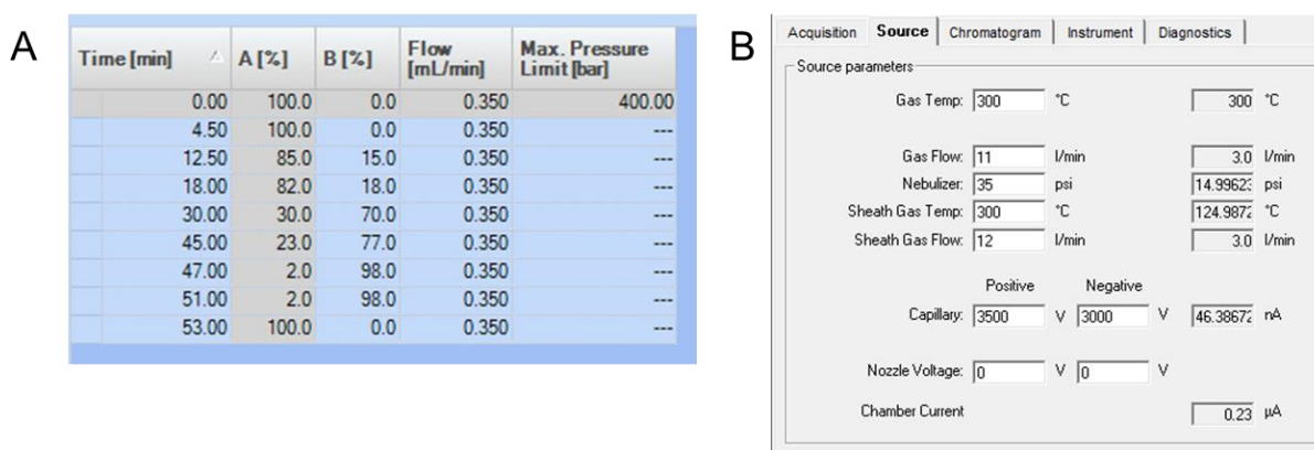
Figure 5.14 LC-ESI conditions for separation of unknown analytes using IPA/MeOH/water (5:1:4) with 5 mM ammonium acetate and 0.1 % acetic acid (Pump A), IPA/water (99:1) with 5 mM ammonium acetate and 0.1 % acetic acid (Pump B), and the gradient reported in (A). The source conditions are reported in (B).
