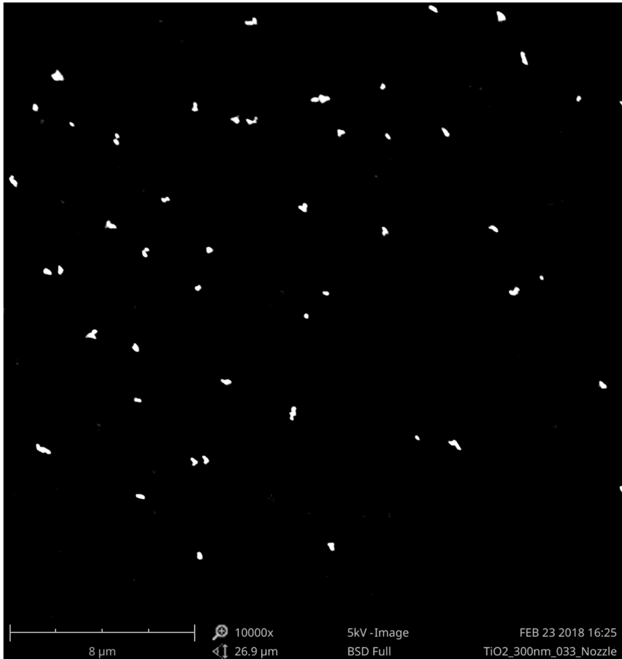
Figure 60. TiO 2 Seeder Sample for 0.85 mm Orifice SEM High Magnification
