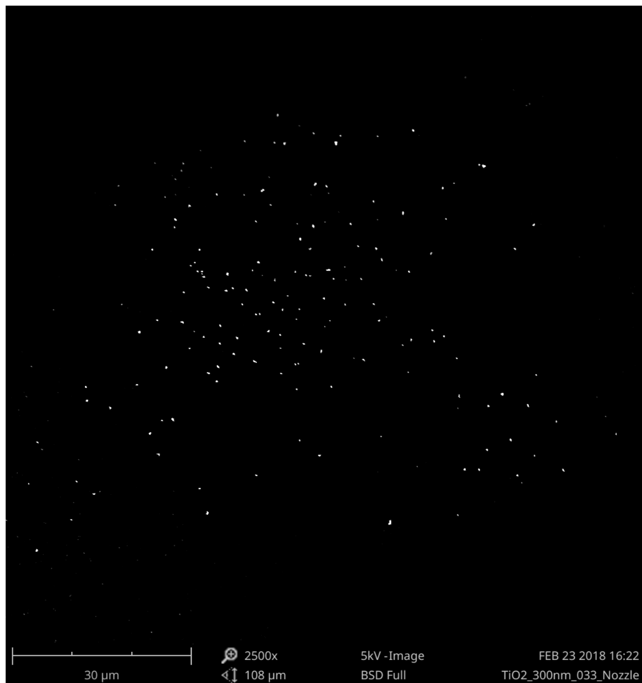
Figure 59. TiO 2 Seeder Sample for 0.85 mm Orifice SEM Wide View
