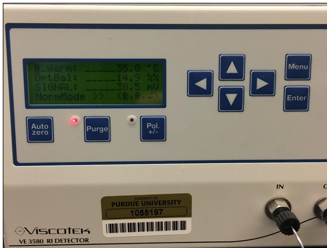
Figure B- 4 Image of RI detector in purge mode
