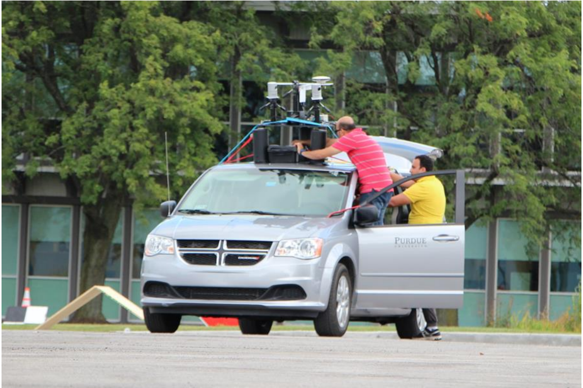
(a) Mounting of LiDAR unit
