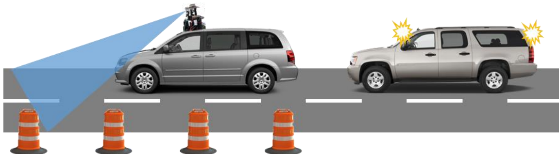
Figure 53 Two-vehicle deployment for LiDAR data collection
