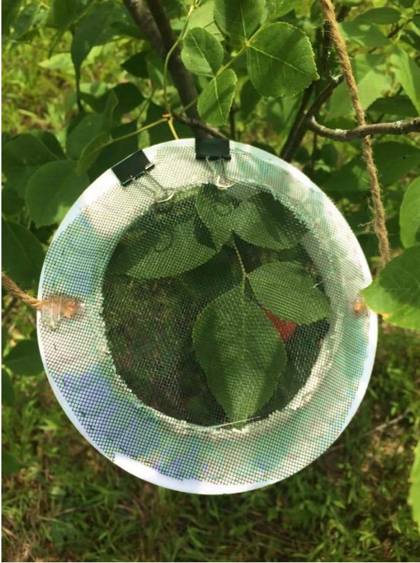
Figure 2.1 Cage used in adult EAB bioassays in 2017. A 10.9 cm diameter section was removed from the center of two 18.6 cm foam plates (Walmart, Bentonville, AZ), which were then stapled together, leaving an 8 cm opening between plates. Two pieces of screen mesh (14.5 x 14 cm) were hot-glued over the opening, and two pieces of 1 m clothesline cotton cord or jute twine (Walmart, Bentonville, AZ) were stapled on.
