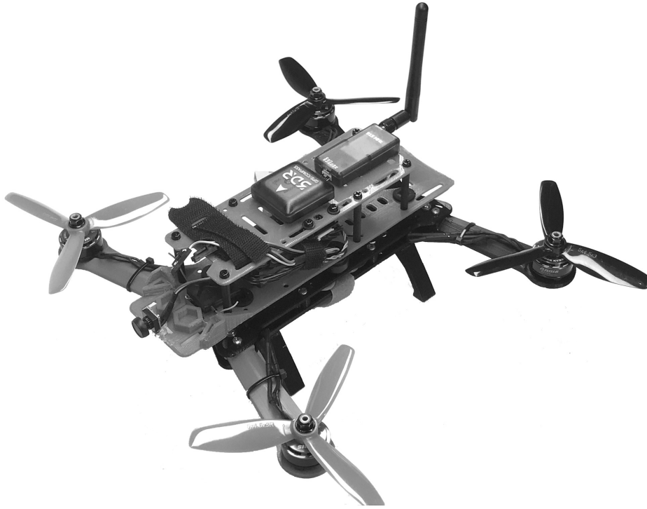
Figure 3.1. MHQ250 drone designed and built for experimental purposes. Original frame design sourced from Thingiverse.com (2014).
