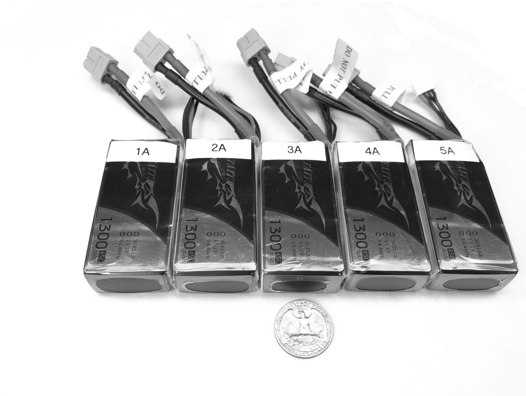
Figure 3.5. Brand new 1300 mAh, 3S1P, 45C rated lithium polymer batteries used in the experiment.
