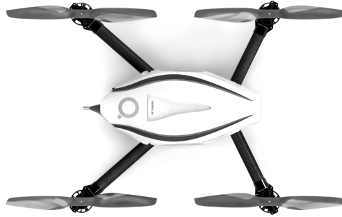
Figure 2.1. Hybrix, a prototype quad-rotor which utilized a series hybrid propulsion configuration (Quaternium, 2015).
