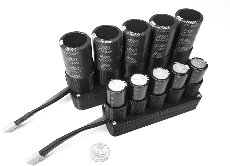
Figure 3.9. 80F5S1P and 20F5S1P supercapacitor arrays purposely built for the experimental test. The smaller sized configuration was the 20F5S1P supercapacitor array. A quarter was shown for size reference.
