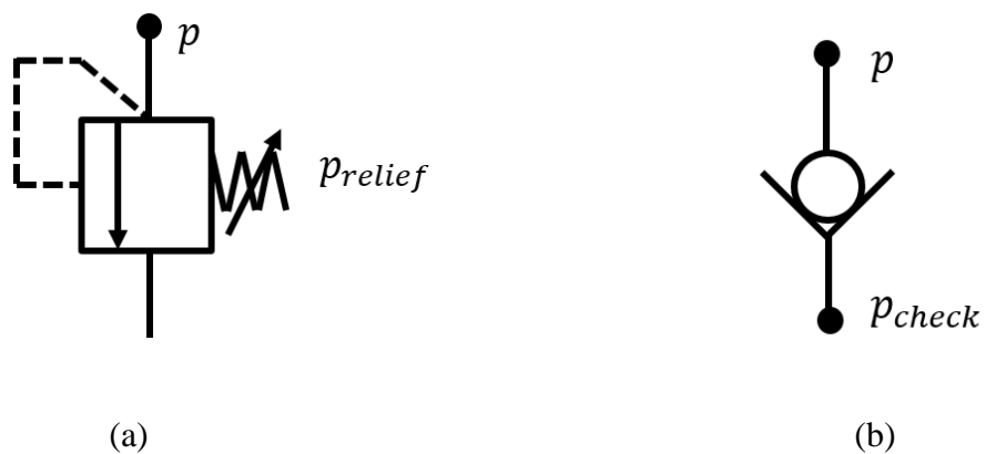
Figure 13. Hydraulic circuit symbols of valves, (a) pressure relief valve and (b) check valve.
