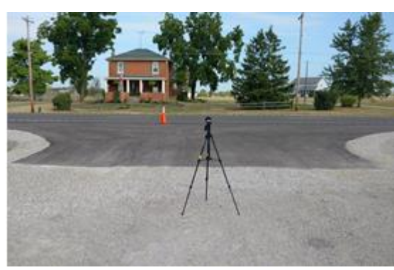
(c) Sound meter at distance of 50ft off the edge line and at a height of 4ft
