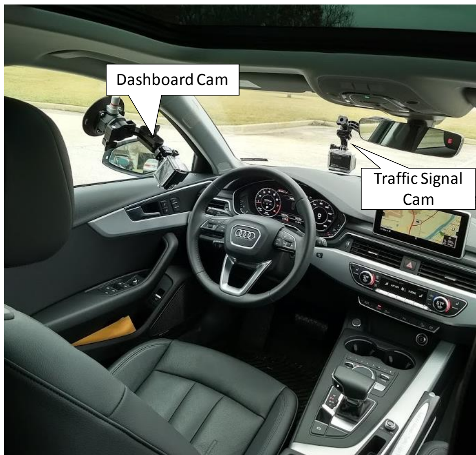
Figure 86. Video camera setup for data collection
