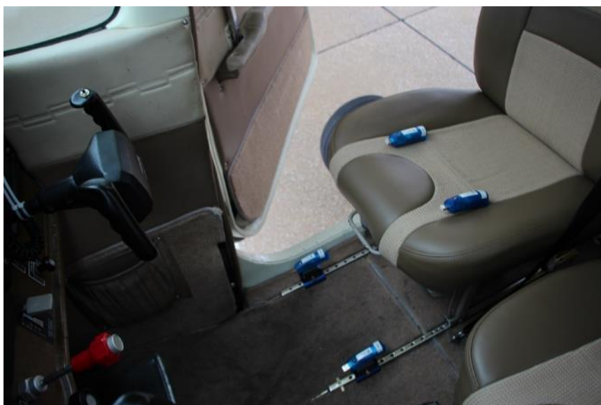
Figure 20. Seat and rail mount configuration on a Cessna 172
