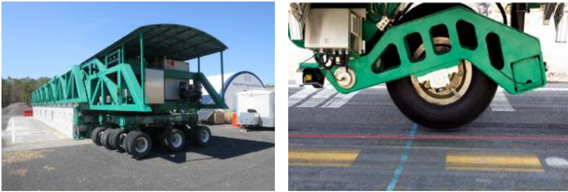
Figure 21. FAA airfield heavy vehicle simulator
