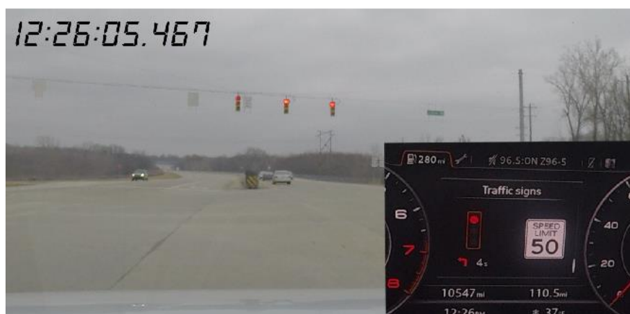
(a) Final red signal countdown time (4s) before it disappears at 12:26:05.467
