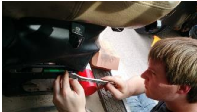
(a) Installing accelerometer on driver side seat frame
