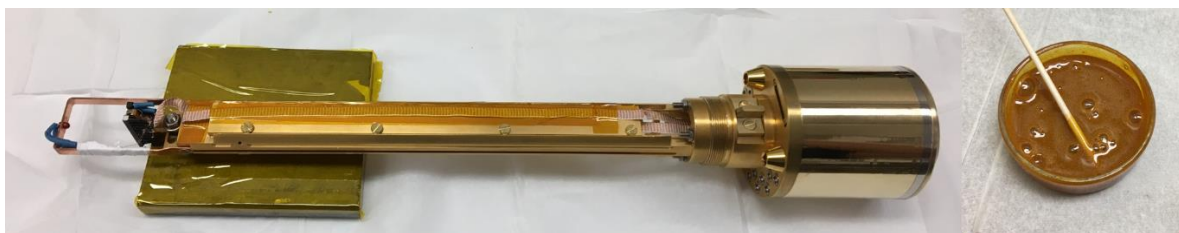
Figure 2.6 new clamping puck with GE-Varnish and silver powder mixture. Left, new clamping puck with copper loom passed through clamp and mixture of GE-Varnish and silver powder coating the copper loom and on the right is freshly mixed GE-Varnish and silver powder slurry
