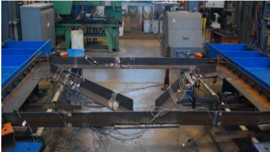
Figure 17 Buckling of the single angle K-frame from Wang[26]
