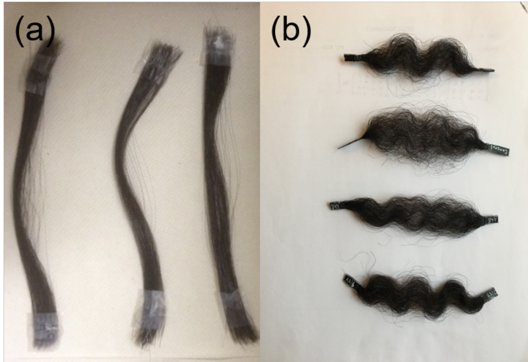
Figure 3.19. (a) Representative prepared bundles of Asian hair. Each bundle contains approximately 30 mg of hair, and the thickness and width are approximately 0.22 mm and 10 mm, respectively. (b) Representative prepared bundle of African hair. Each bundle contains approximately 30 mg of hair, and the thickness and width are approximately 0.5 mm and 10 mm, respectively.
