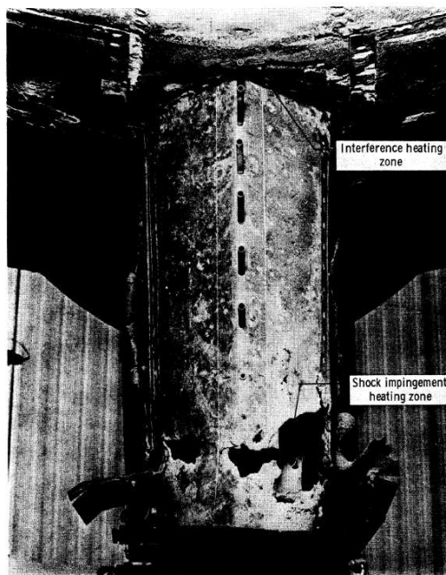
Figure 1.1. Damage due to shock impingement on the X-15 pylon [1].
