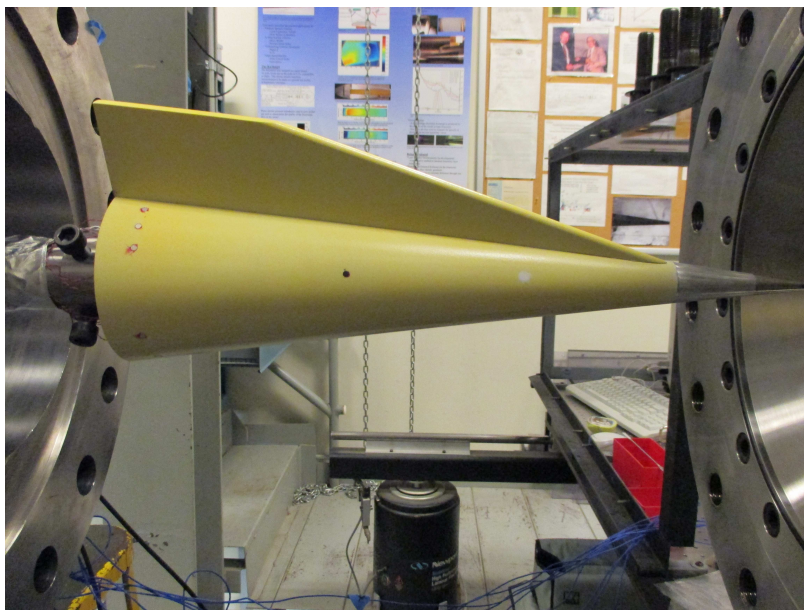
Figure 3.7. Model ready to install in tunnel with TSP applied.
