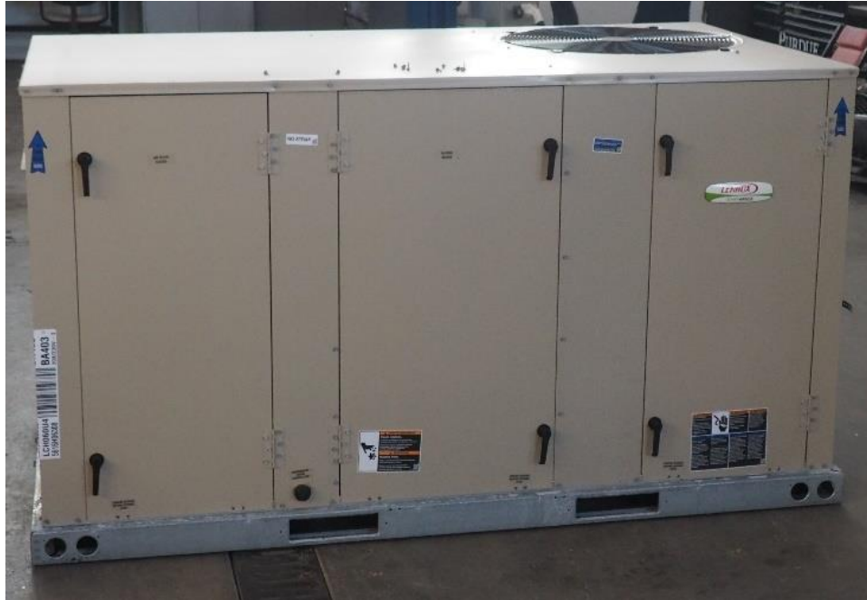
Figure 2.10. 5-ton variable-speed RTU that will be used to develop and evaluate AFDD implementation.
