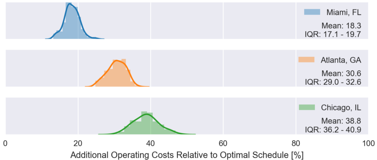
Figure 6.31. Additional lifetime operating costs relative to optimal lifetime costs when biennial service schedules are used to service multiple faults in three different locations.
