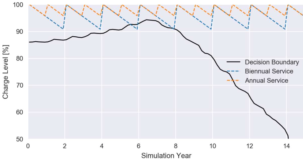
Figure 6.11. Comparison of lifetime refrigerant charge levels for system located in Miami, FL with a leakage rate of 5% percent per year using biennial and annual periodic service schedules.
