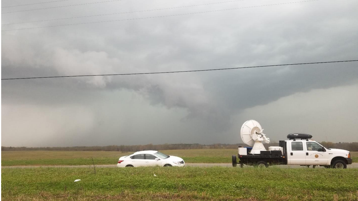
Fig. 16. UMass X-Pol next to a white car with the leading edge of a thunderstorm in the background. Photo captured by the author on 27 March 2017 1903 UTC in Killen, Alabam.
