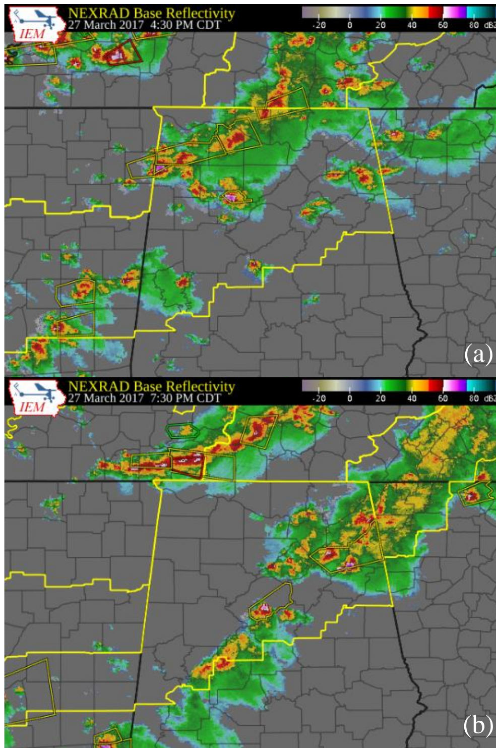
Fig. 25. Mosaic of NEXRAD base reflectivity (in dBZ) for 2110 UTC 27 March 2017 (a) and 0010 UTC 28 March 2017 (b) over the VORTEX-Southeast domain. Thick yellow lines enclose SPC-issued severe thunderstorm watches. Smaller yellow, red, and green polygons enclose NWS-issued severe thunderstorm, tornado, and flood warnings, respectively. Images obtained from the Iowa State University Iowa Environment Mesonet (ISU IEM) website.
