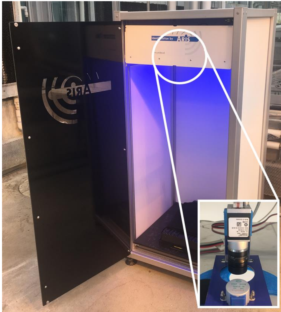
Figure 8. Top-view image station (Aris B.V., The Netherlands) where leaf area of plug trays was estimated non-destructively.
