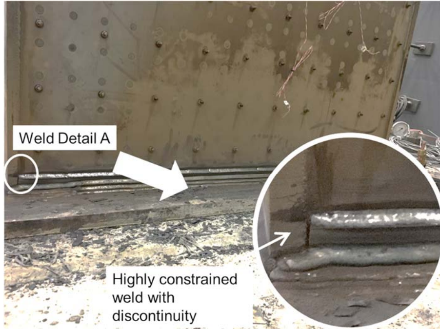
Figure 6.26. SC-W-H: Faceplate-flangeplate-baseplate weld detail
