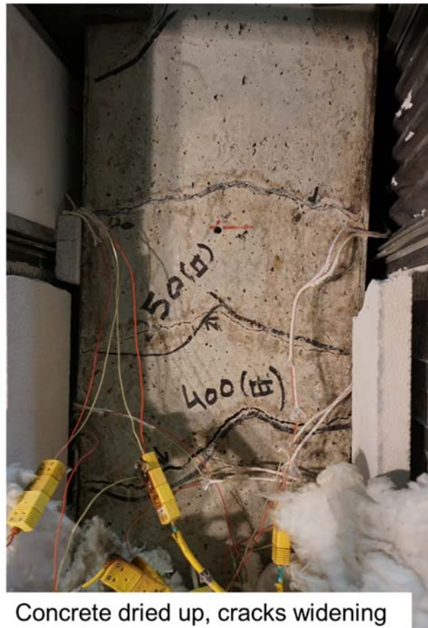
Figure 6.13 SC-WP-H: Specimen state (South face) at 1.5\Delta_y -232°C-1 hour cycle (cycle no. 10)
