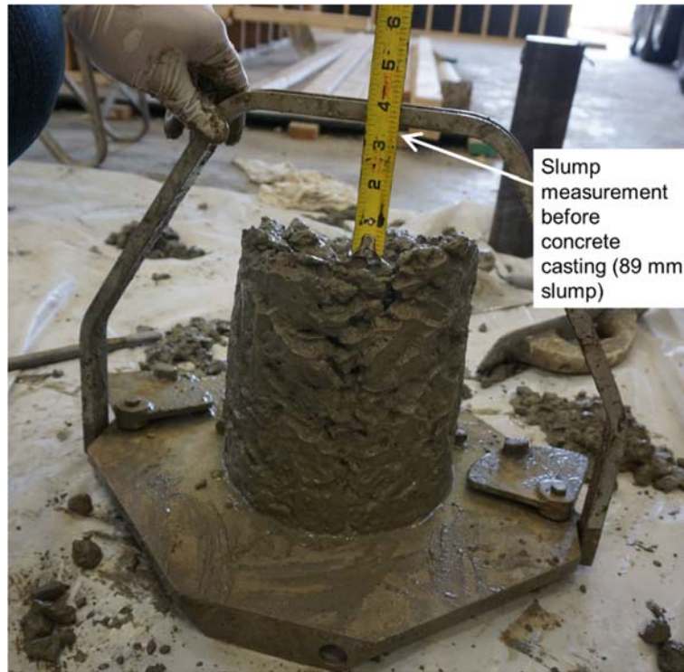
Figure 5.23 SC-WP-H: Measurement of slump before concrete casting
