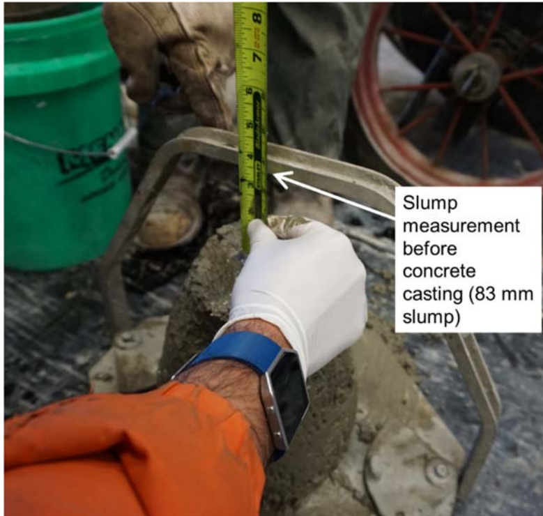
Figure 5.29 SC-W-H: Concrete slump test before casting
