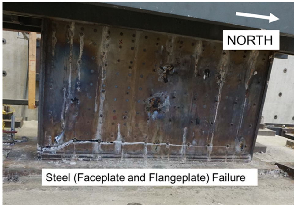
Figure 6.30 SC-W-H: East view of specimen after failure (failed during 3\Delta_y push cycle)
