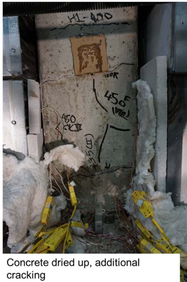
Figure 6.12 SC-WP-H: Specimen state (North face) at \Delta_y -232°C-1 hour cycle (cycle no. 8)
