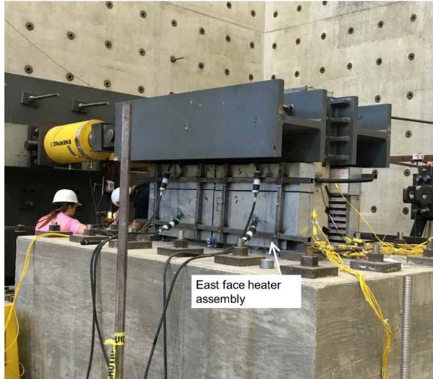
Figure 5.25 SC-WP-H: Heater assembly installed
