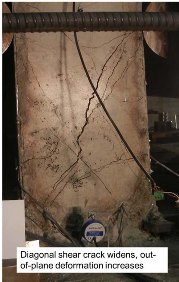
Figure 4.46 SC-T-2.5Vn: Specimen state (North face) at \Delta_y , pull cycle 1
