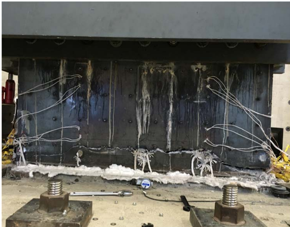
Figure 6.16 SC-WP-H: Specimen at failure (faceplate rupture)
