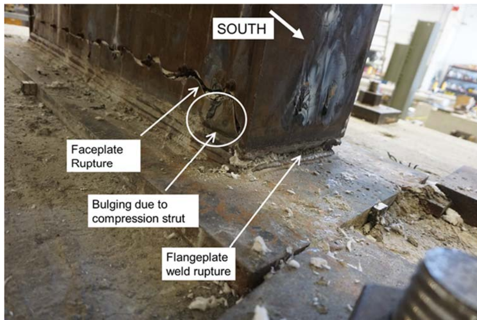
Figure 6.31 SC-W-H: South-West view of specimen after failure (failed during 3\Delta_y cycle)
