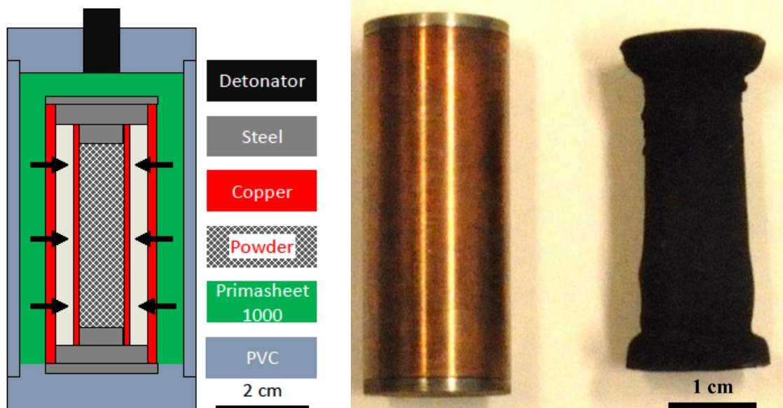
Figure A.1. Concentric cylinder powder compaction experiment as well as an image of the capsule before and after shock.
