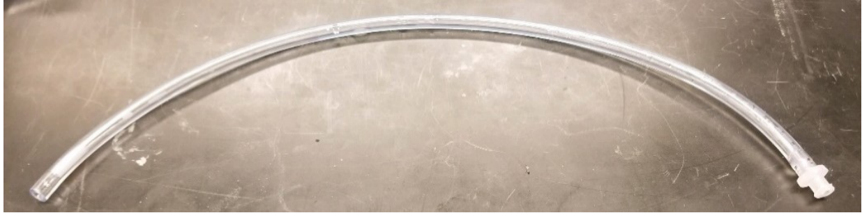
Figure 4.10: 14-inch long, 3 mm diameter tubing, connecting the pumps to the test sections.
