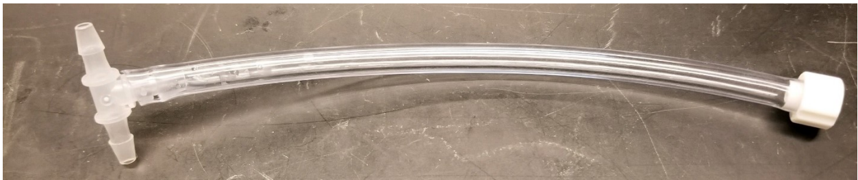
Figure 4.8: 3 mm tubing with a stopper on the end, used to dampen the perturbations produced by the rollers in the peristaltic pump.
