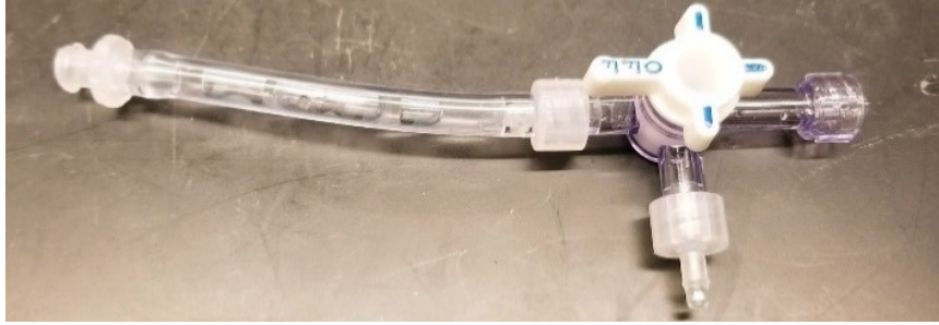
Figure 4.7: The three-way valve, and 3 mm diameter tubing, which connect the syringes to the test sections. Tubing leading to the pumps is not shown.
