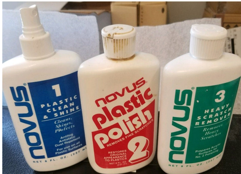
Figure 4.1: Stage 1-3 of the Novus brand polishing solutions used on the acrylic test sections.
