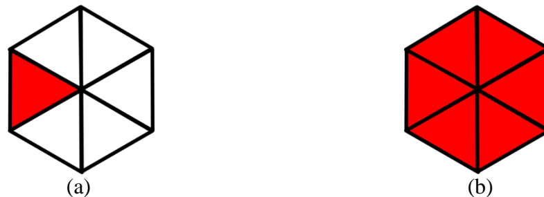
Figure 3.16: Types of initial voids randomly placed in the microstructure topology region (a) small void and (b) large void. Elasticity modulus of elements colored in red is set to 0.
