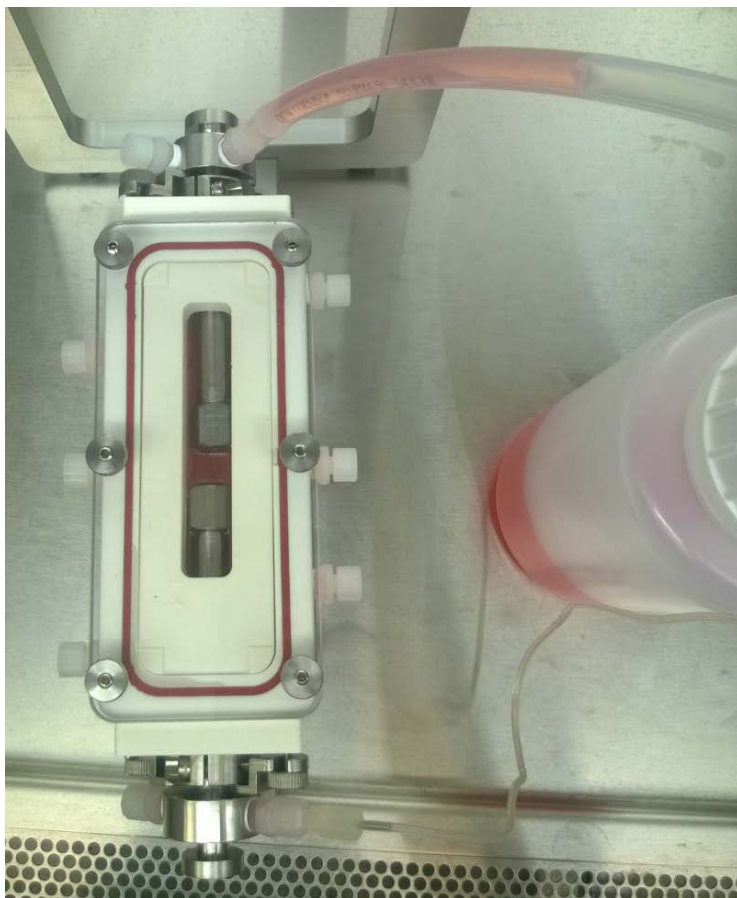
Figure 5.1 Image showing the flow loop between the reservoir bottle and the chamber.
