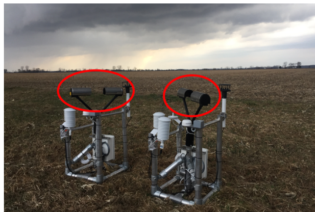
Figure 1. A photograph of two PIPS, complete with disdrometers and weather sensors. The Parsivel 2 disdrometers are circled in red.
