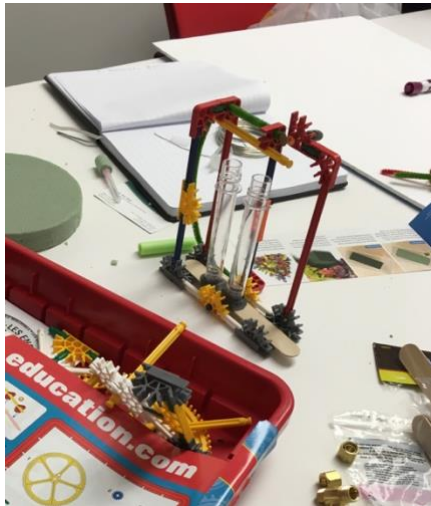
Figure 49: Low-fidelity prototype of fluid collection system using K'NEX tongue depressor, plastic tubes, and clay.
