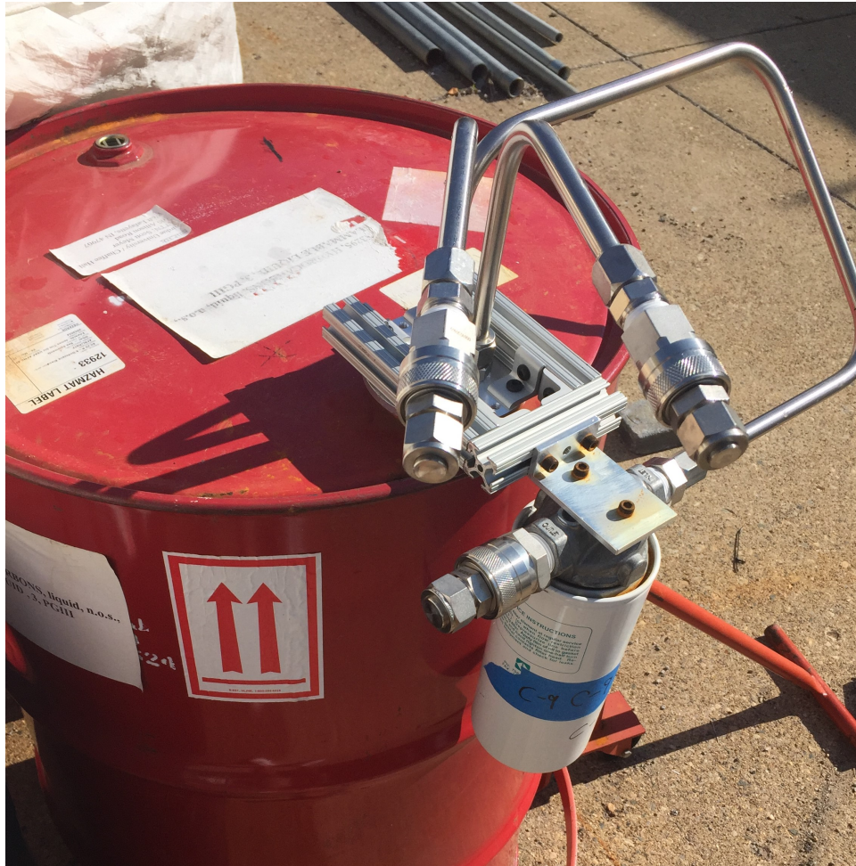
Fig. 3.8.: Fuel manifold assembly connected to fuel drum
