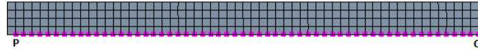
Figure 3.7.: Line of nodes chosen for comparing contact stresses on the upper cantilever beam
