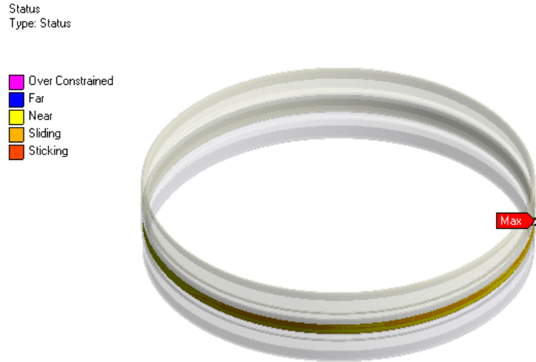
Figure 3.30.: Interlock contact status
