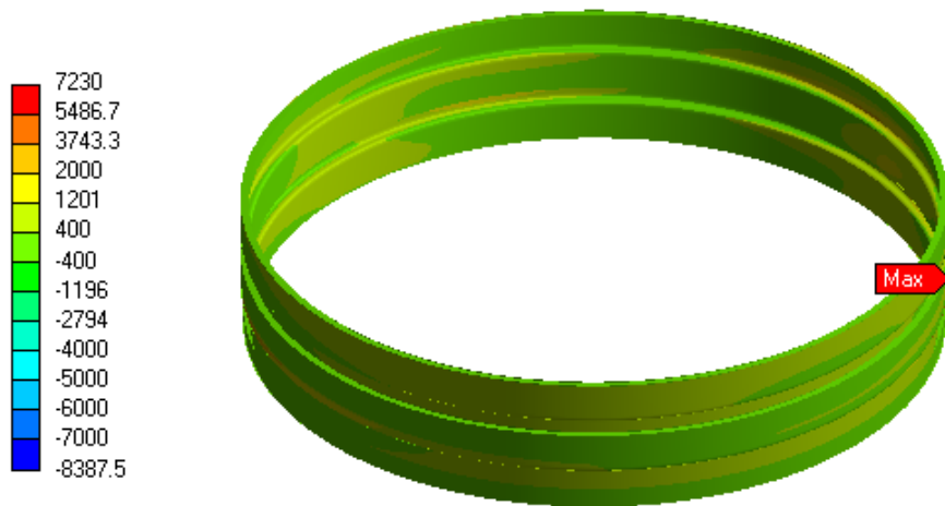
(b) Maximum principal stress - interlock simplified
