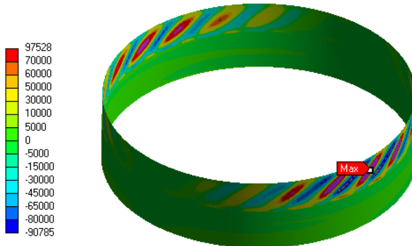
(b) Normal stress - concentric ring simplified
