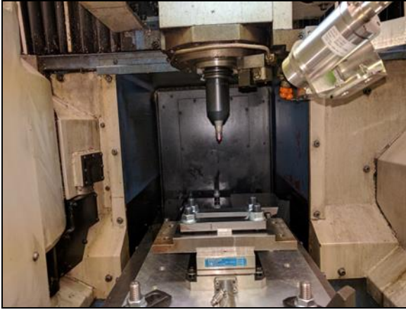
Figure 4-1: Experimental Setup of FSSW on Al 60601-T6 plates.
