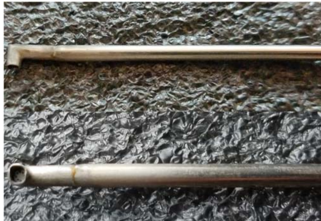
Figure 2.8: Kulite LQ-062 pressure transducer installed in Kiel head probe.
