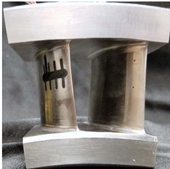
Figure 2.7: Removable stator vane passage insert instrumented with Kulite LQ-062 pressure transducers.
