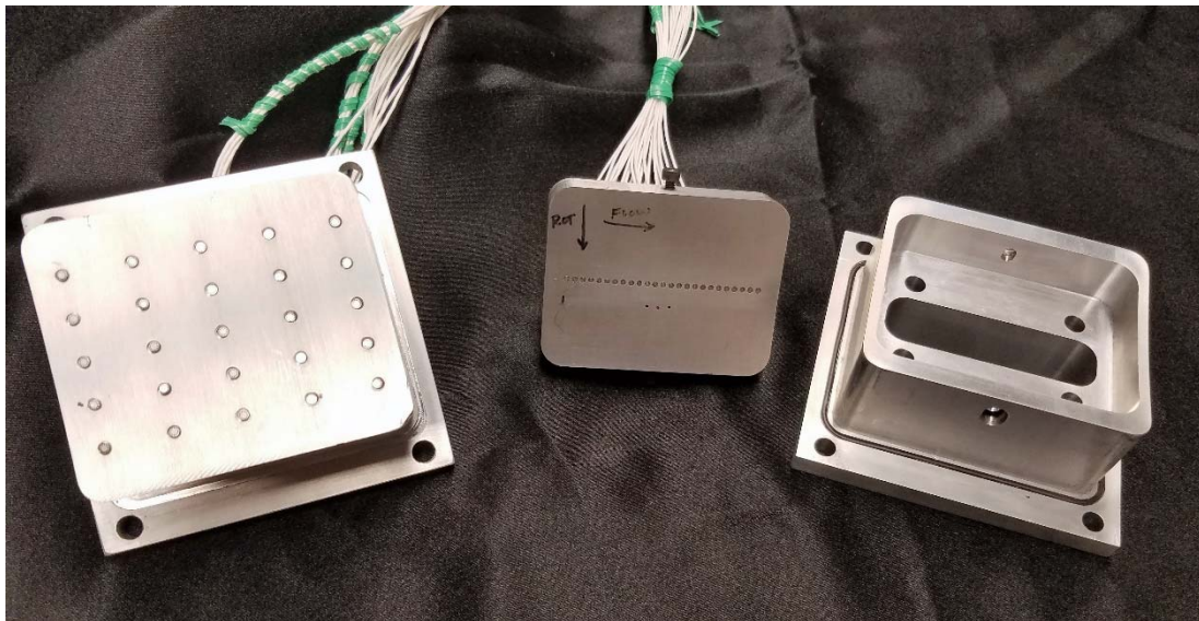
Figure 2.5: Instrumented blocks for over-rotor endwall static pressure measurements.
