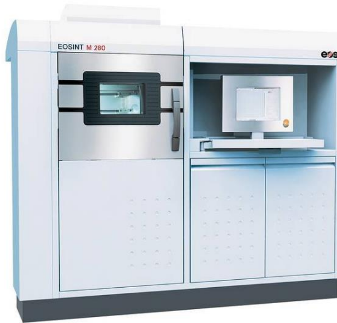
Figure 17: EOSINT M280 high definition additive manufacturing system [103]
