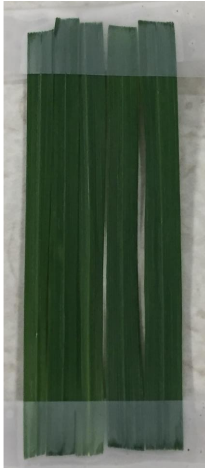
Fig. 4.1. Example of a leaf mat. The leaves are arranged to fill the field of view of the plant probe used to measure the reflectance of each plant.
