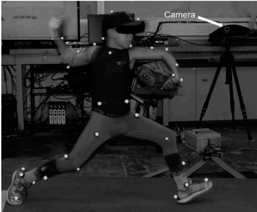
Figure 1. Participant pitching a portable pitching mound with retro-reflective markers to capture kinematic data with one of 10 motion analysis cameras shown.
