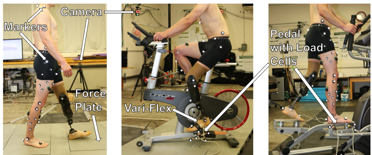
Fig 1. Setup for gait, cycling, and elliptical training motion analysis experiments. Digital cameras, ground force plates, reflective markers, the Vari-Flex prosthesis with foot cover, and instrumented exercise machine pedals are indicated.
