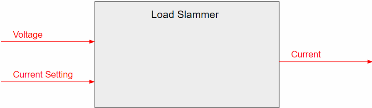
Figure 3- 2: Level 0 Block Diagram for Load Slammer
