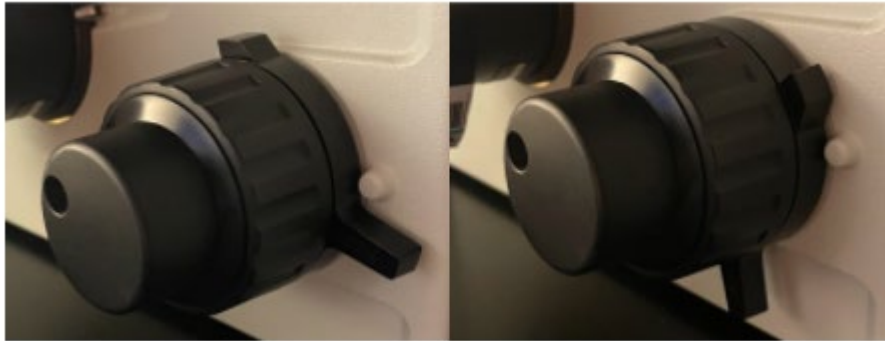
Figure 8. The stage adjustment knob unlocked (left) and locked (right).
