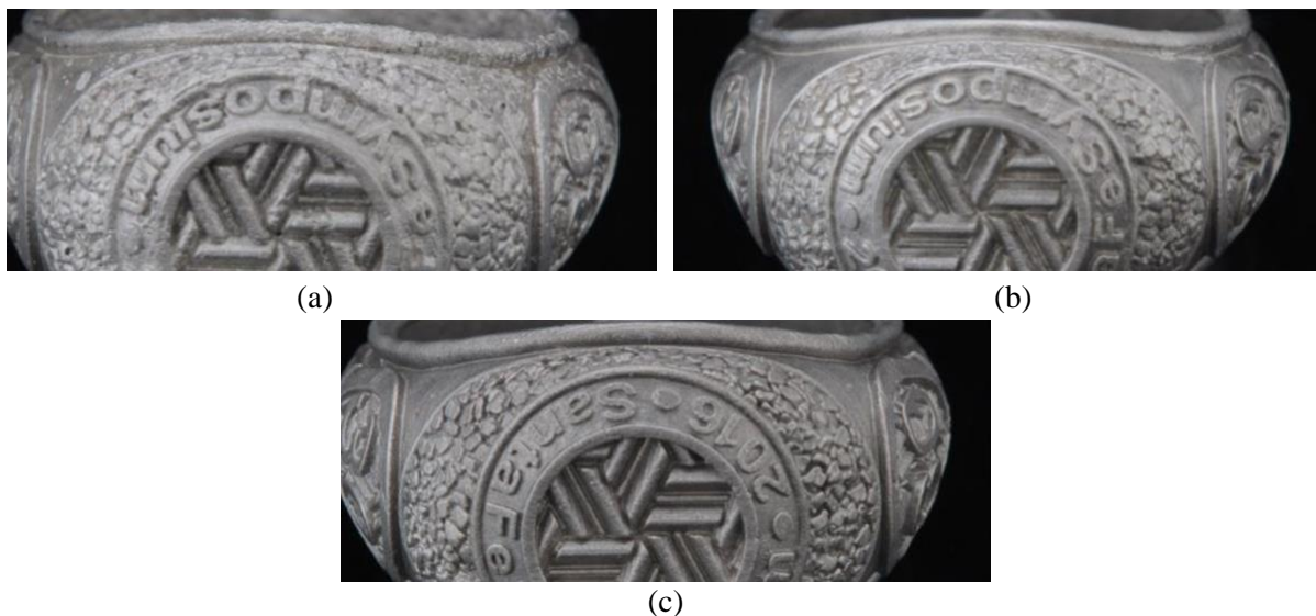
Figure 3. Three identical models with different curing methods. (a) had the standard UV cure, (b) had a heated cure, and (c) had a heated cure in a vacuum. The images show the increase in quality from the UV cure to the vacuum-heated part [6].
