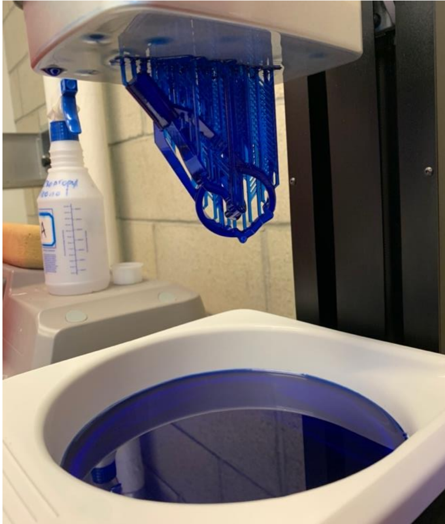
Figure 32. These interlocking rings came out well, as they stuck to the build plate and had no failures prior to burnout. By angling the part, it reduces the adhesion area on the florescent surface and thus has a lower chance of failure.
