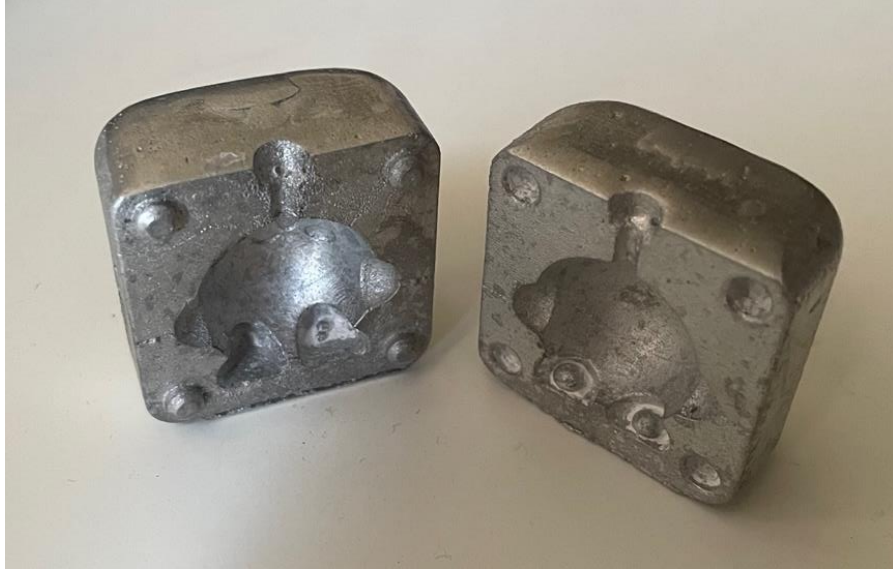
Figure 38. The other example model we wanted to prepare was the Kirby action figure, but instead we changed this to a die-cast model. As shown, the Kirby figure is a cavity that when the two pieces are clamped together, can be filled with hot glue/liquid wax and allowed to harden. This was created to show the students a different form of manufacturing and how dies can be cast instead of machined.
