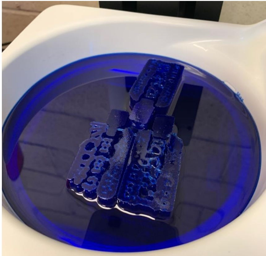
Figure 31. As seen, this print prematurely separated from the build surface. This was because the print wasn't angled at 35°, which has been shown to produce a good quality print with less likely chances of peeling failures.
