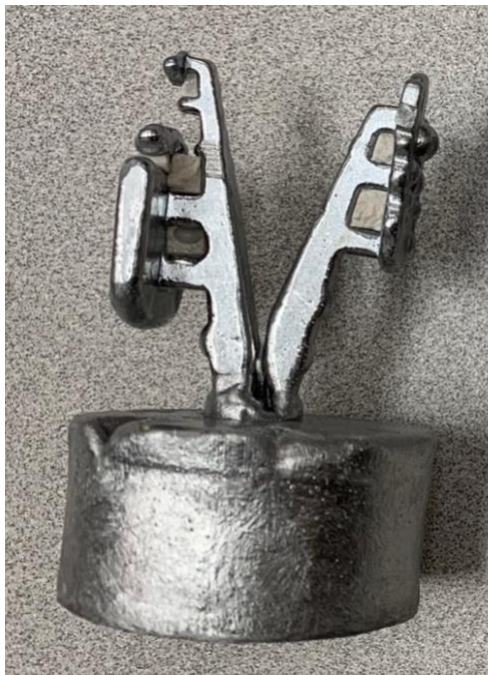
Figure 38. As seen, the metal barely got through the sprues since it didn't have the vacuum pressure drawing it into the cavity.
