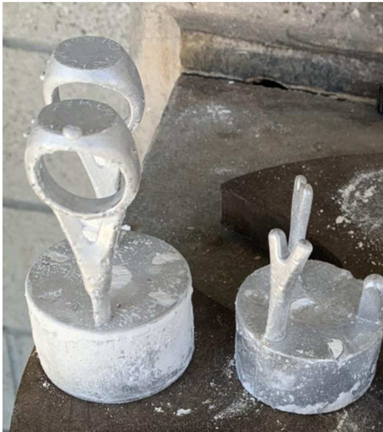
Figure 41. On the right, a successful cast that was done under vacuum pressure. On the left, the flask had cracked, and the metal only halfway made it down the sprue under a gravity-pour. To improve success, a vacuum pump could be used during investment to prevent the flask from cracking due to air pockets in the plaster.
