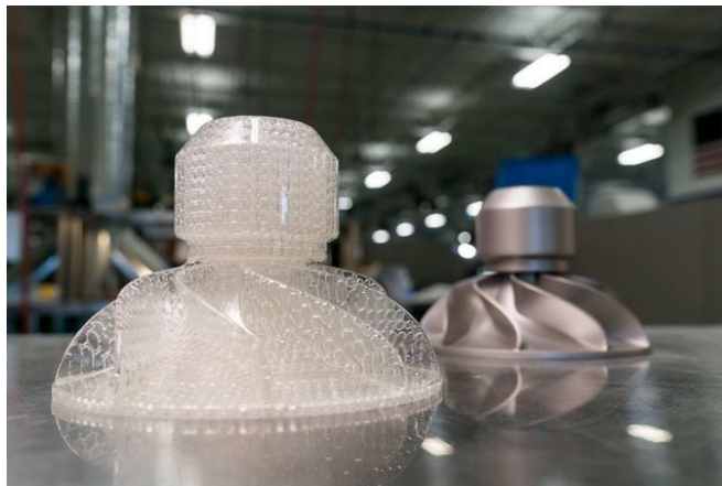
Figure 1. A 3D printed resin pattern (left) used to cast the investment casted part (right) [1].
