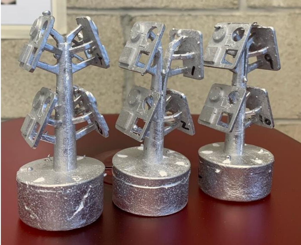
Figure 35. A new test coupon was created for statistical measures that has much fewer features to document. 12 of these were produced for a large enough sample size to accurately document the shrinkage rates.
