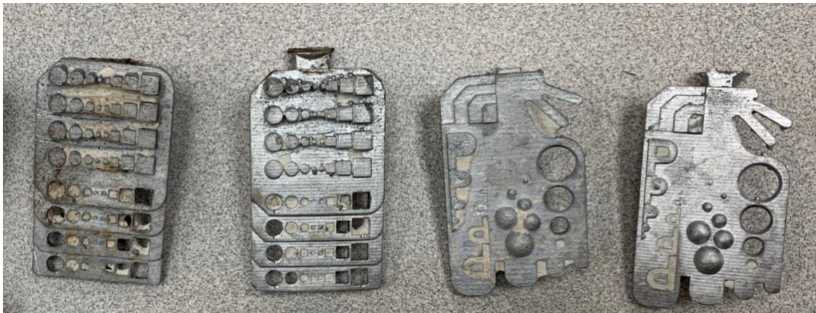
Figure 34. A few of the casted coupons. In total, 5 of each test coupon were successfully cast and used for analysis on the limitations of sizing (minimum thicknesses or diameters). These hadn't been fully washed prior to the image, and thus the reason for residual plaster to be stuck between features.
