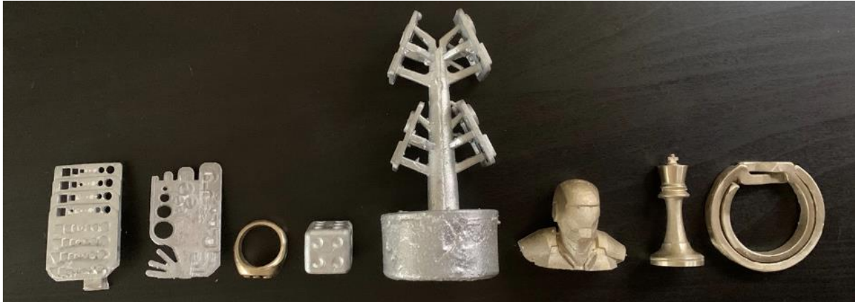
Figure 40. Successful models from left to right: test coupon A, test coupon B, ring, dice, new test coupon, iron man bust, chess piece, interlocking rings. There were a total of 8 successful pieces from the original design. Additionally, the Kirby die was successful, as shown in Figure 38. The Kirby, ring, and dice account for the three student models that were requested.
