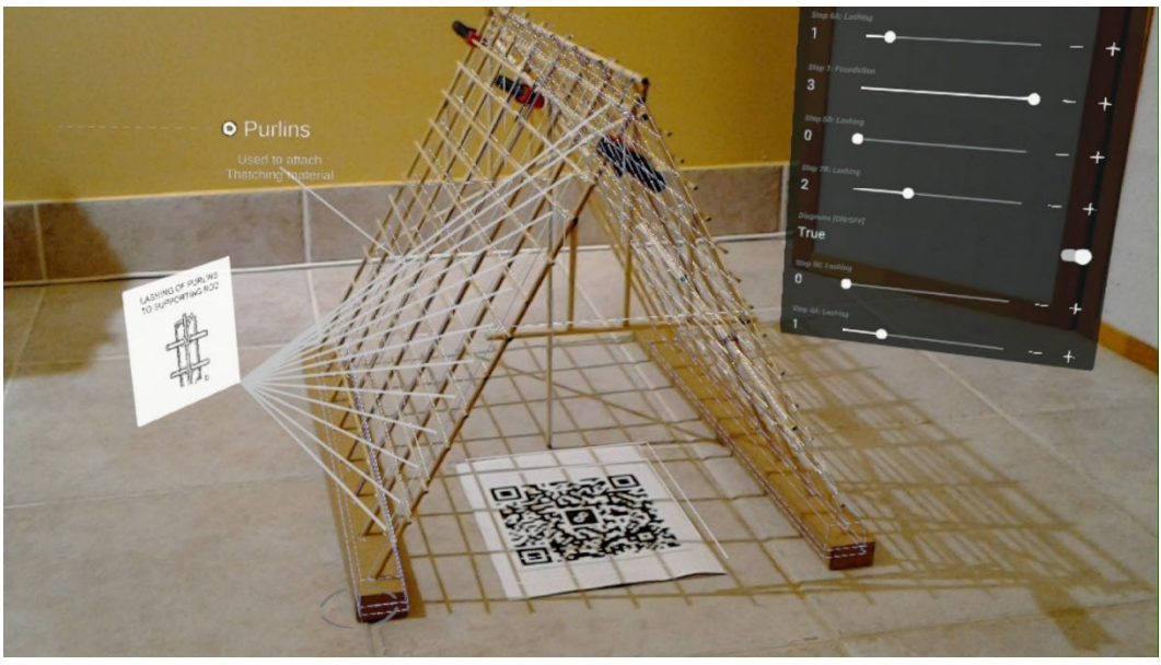
Figure 58. Placement of Vertical Purlins Over the Horizontal Purlins
