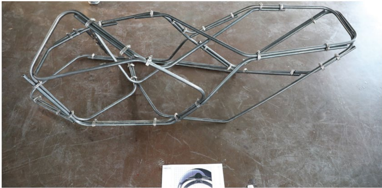
Figure 26. A Small Chunk of the Pavilion with Image Marker Used to Calibrate Digital and Physical Models During Digitization
