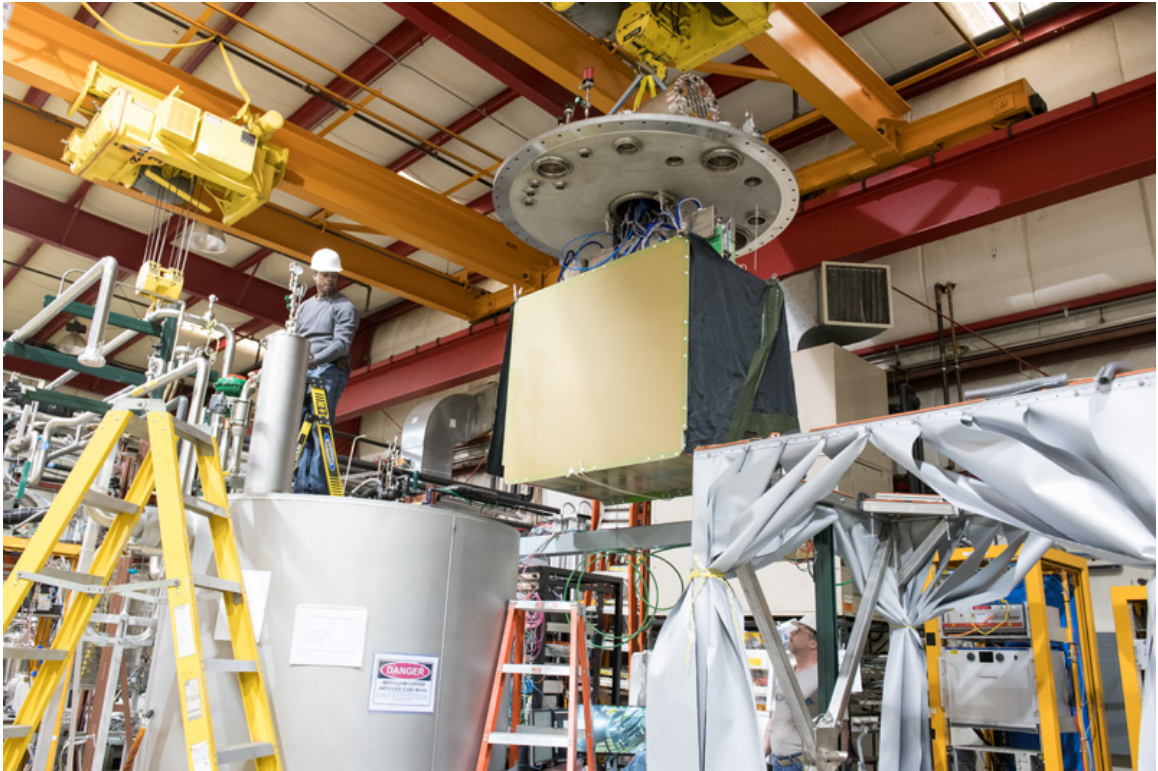
Figure 2.1 Fermilab's ICEBERG test bed is effectively a miniature version of the component that tracks neutrinos in the international DUNE experiment. ICEBERG is used to evaluate performance of potential components of DUNE.
