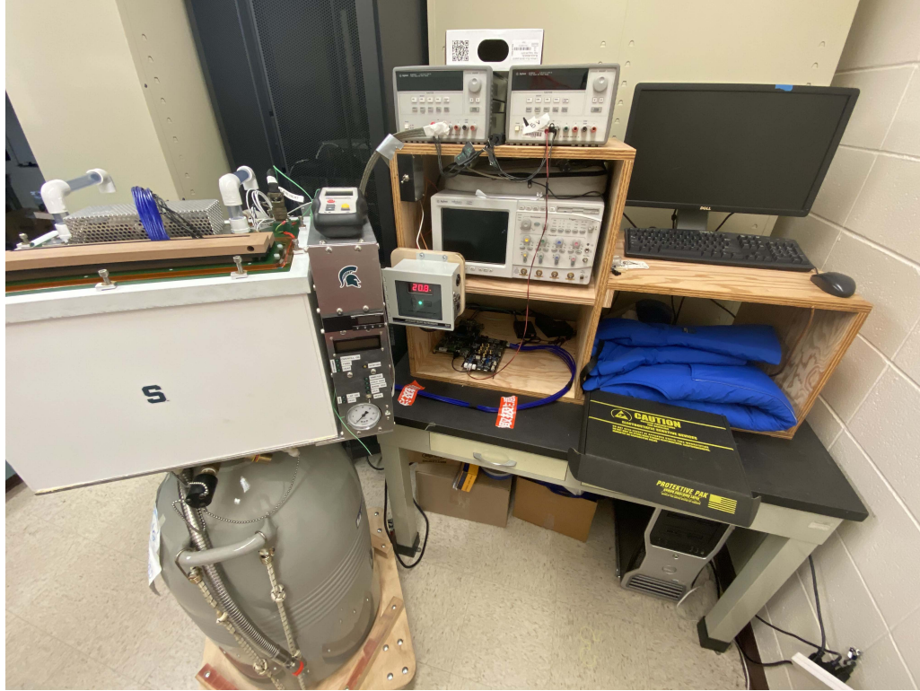
Figure 4.1 Lab space for the communication and testing of the FEMB. CTS unit on left allows shielding and submergence into liquid nitrogen. Power supplies on top for multiple voltage rails. Scope and multi meter for debugging signals. Linux interface on the right.
